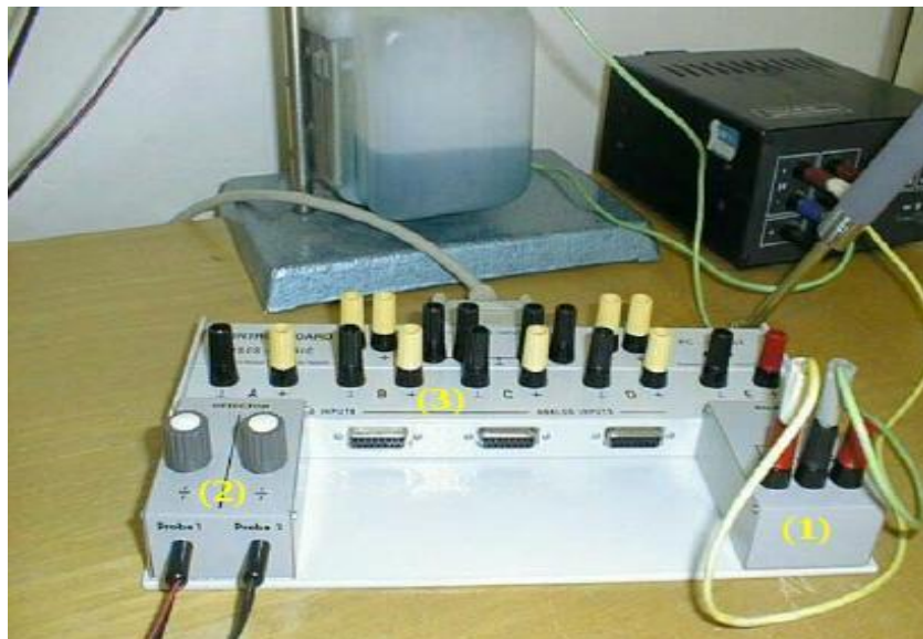
Figure 1 – Location of the control remote experiment controlling the water level Relays (1), Sensors (2) and ISES Panel (3)
